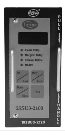
USE THE ADAPTER HANDLE (NOT THE AMPLIFIER HANDLE) TO REMOVE THE ADAPTER/AMPLIFIER ASSEMBLY FROM THE WIRING RACK
